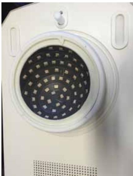
**Figure 2.** The scanner consists of an array of radio antennas arranged around the inside of a hemispherical bowl. The array is located below a hole in the scanner bed and is covered by a round cup that fits the breast when the patient is in the prone position
