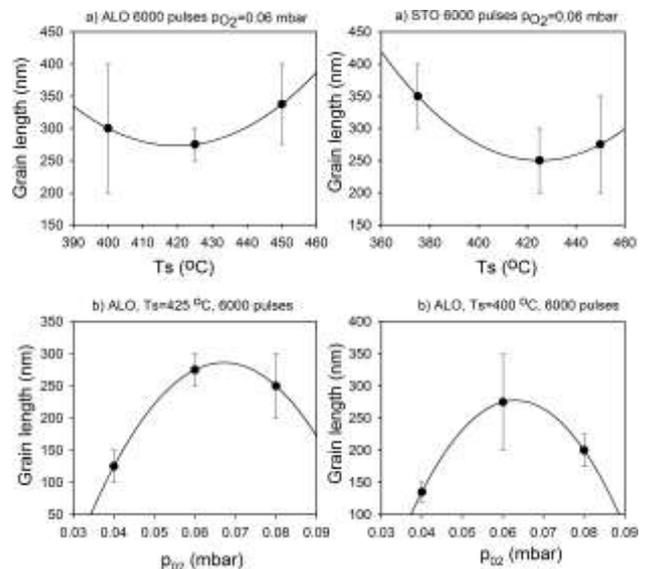
**Figure 6:** Dependence of the grain length on a)  $T_s$  for ALO and STO substrates and b)  $p_{O_2}$  for ALO substrate. Lines are just guide for the eye. Bars indicate uncertainty in value.
