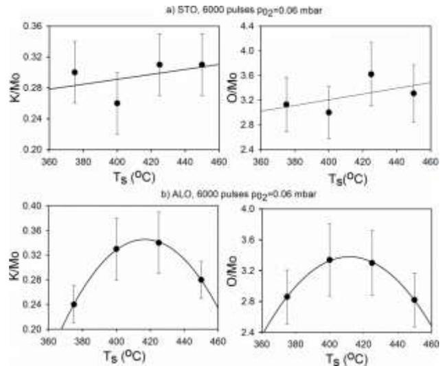
**Figure 5:** Ratio of K/Mo and O/MO atoms vs.  $T_s$  for a) STO and b) ALO substrate. Lines are just guide for the eye. Bars indicate uncertainty in value.
