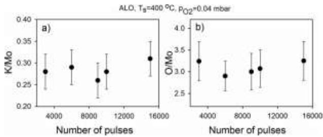
**Figure 3:** Stoichiometry of deposited films vs. number of pulses for ALO substrate: a) ratio of K/Mo and b) O/Mo atoms. Bars indicate uncertainty in value.
